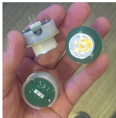
Electronic Voltage and Current Regulator Khatod 10-degree lens and holder. The final optics together with a 3d printed spacer made in my studio.
